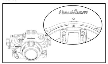
Align the mounting indices of the port and the housing; these appear as white circles on both the port and the housing.
