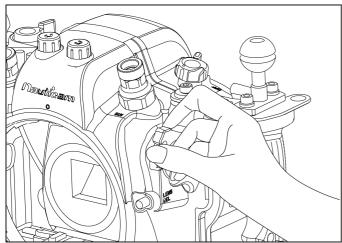
Pull the Zoom/ focus gear disengagement lever before mounting lens (with gears installed) to the camera. Engage the gears by pulling up the lever to the original position. Confirm that the zoom/focus knob operates correctly.
